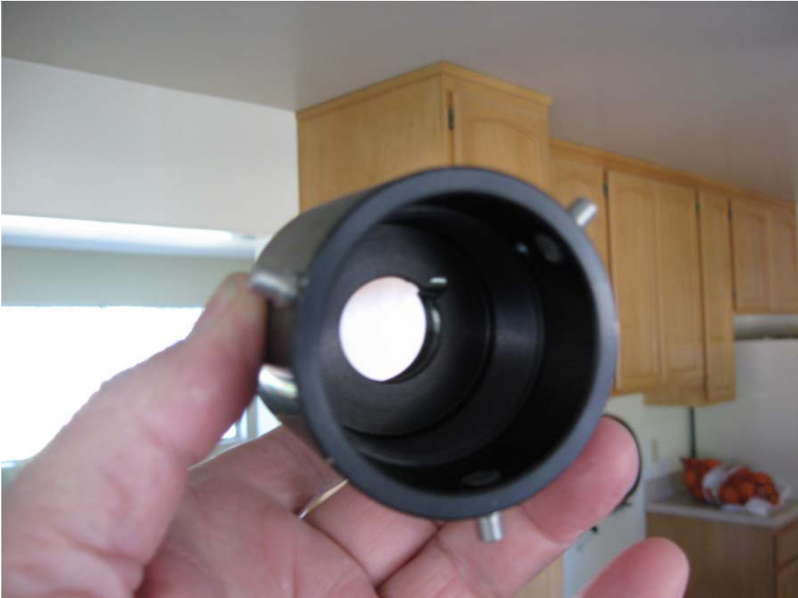
Photometer body with three point mounting
