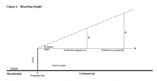
To find the maximum allowable mounting height, take the distance (b) from the property line to the base of the fixture location and multiply it by .47. This will give you (a), the height above the 5 foot starting level. Add (a) to 5 feet to find the maximum allowable mounting height.
