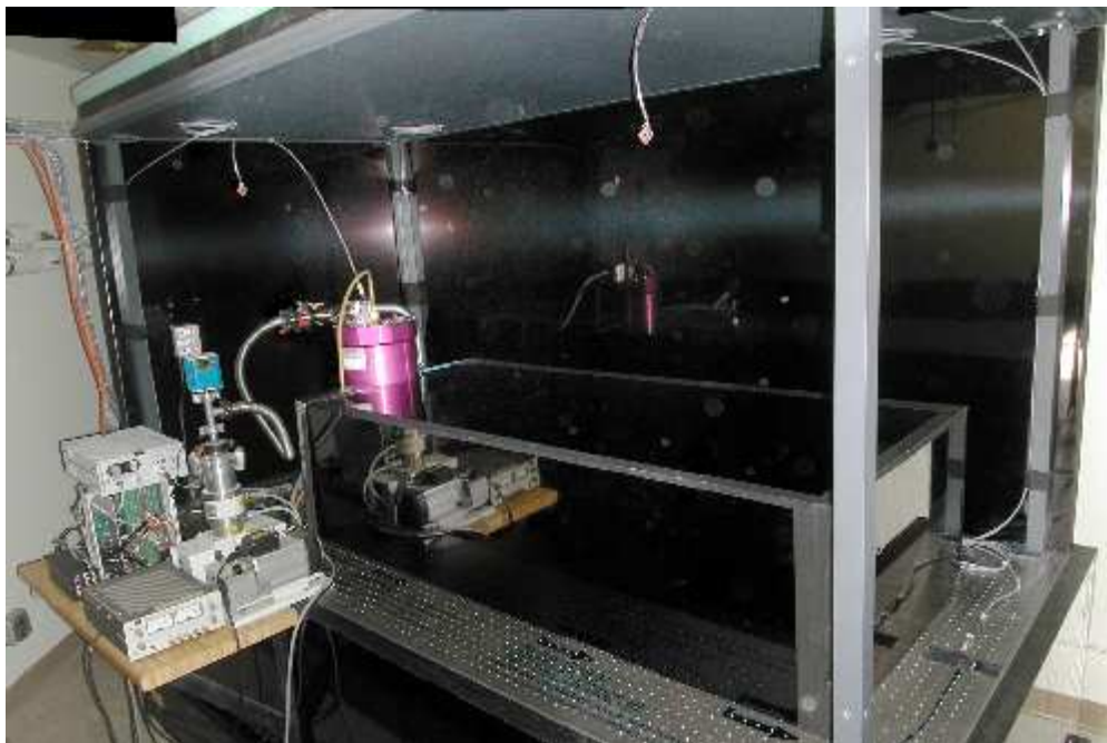
Figure 2.65: Thermal insulation of the optical bench. The optics are covered with a one inch wall thickness black box (aluminum-foam-aluminum sandwich), while the same insulation material in two inch thickness is used to enclose the entire optical bench. sandwich
