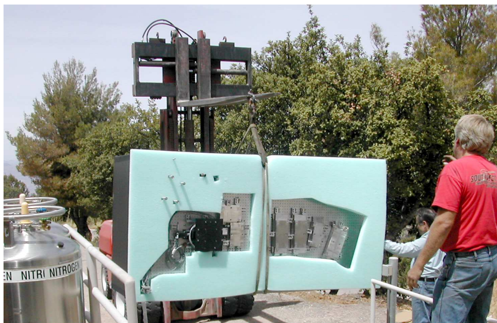
Figure 2.81: The TRES optical bench arriving to FLWO. Note the steel lens mounting bases and focus stage (black) within the cutout of the protecting foam. By securing these blocks, and thanks to the kinematic mounts, no alignment was necessary upon re-assembling the TRES optics.
