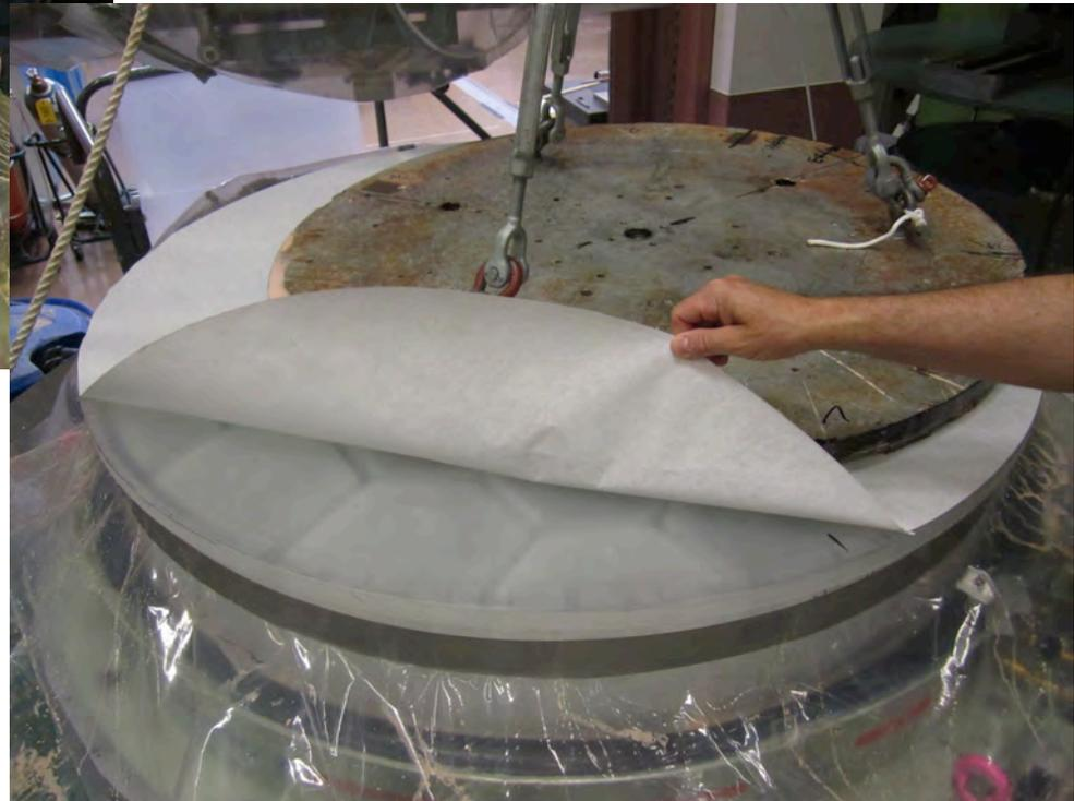
Polishing tool on mirror after the first polishing run.
