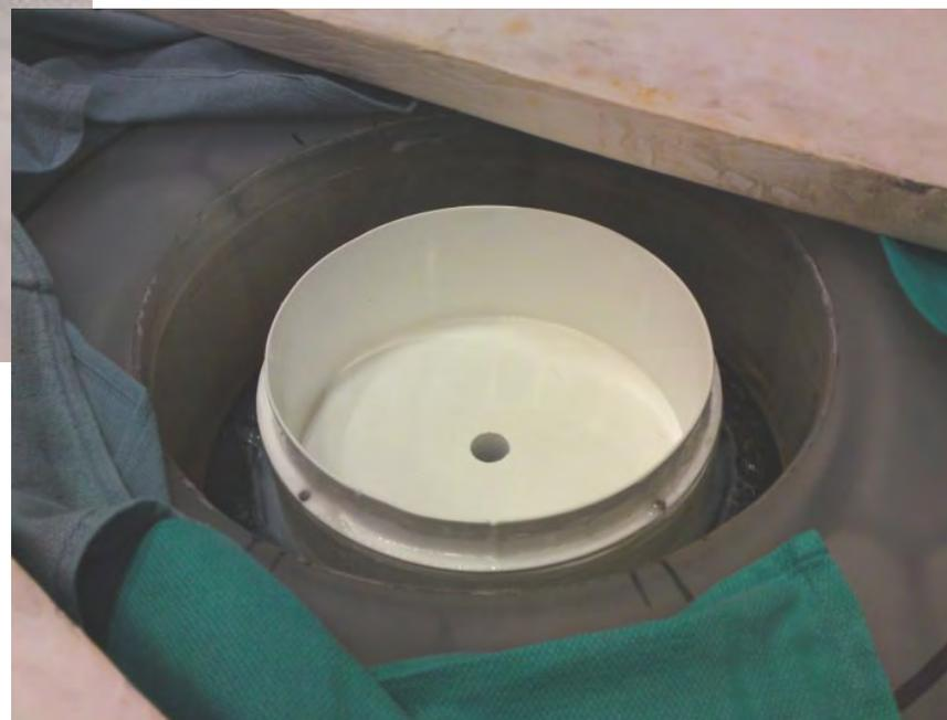
The center hole seal leak due to corrosion. The part was replaced, powder coated and installed.
