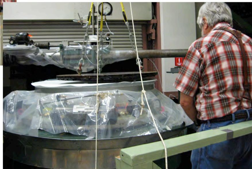
New polishing lap being put on the mirror to be pressed-out prior to the first polishing run.
